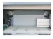
height is 254 mm or 10". Stacked sheets are delivered to the output conveyor for easier handling or downstream finishing.
