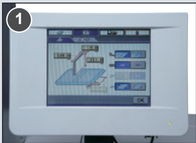
1 Input the dimension of the book block into the touch screen.
