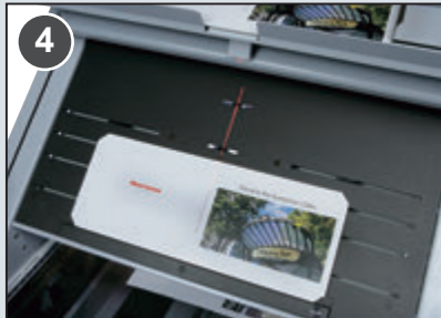
4 Position the adhesive backed cover using the laser center line for accurate print or image alignment.
