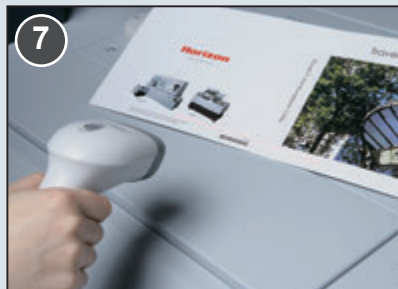
7 Verify a match of the case and book block by scanning the barcode with optional HCB-2BC Barcode verification system.
