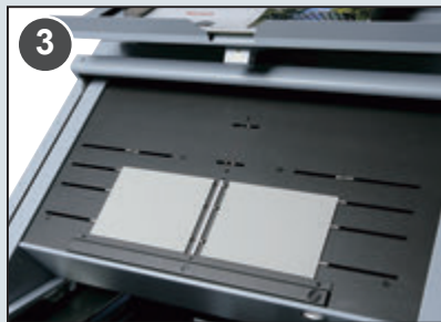
3 Place the card board according to the automatically pre-set positioning guides.
