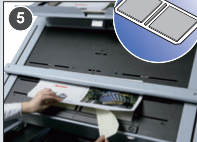
5 Remove the release lining to attach the cover to the card board.
