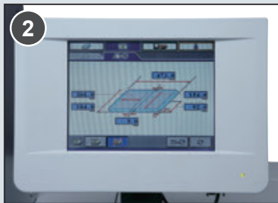
2 Cover size and card board size are displayed on the screen. Corner cutting tool for covers is provided as an accessory.
