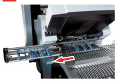
The uniquely designed delivery belt unit can slide out for easy set up of scoring and perforating positions.
