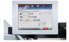
The 12.1 inch color touch-screen is icon-based for user-friendly operation. Each section is automatically set by inputting sheet size and fold pattern. Roller gaps can be adjusted by 5  $\mu$ m (0.005 mm) and the buckle stopper can be adjusted by 0.1 mm / 0.005" at the touchscreen. Up to 200 job settings can be stored in job memory.
