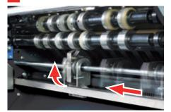
Perforation, slit perforation, scoring and slitting can be performed. Scoring can be positioned easily using the uniquely designed scoring navigator. The position can be saved in job memory for easy recall of repeated jobs.
