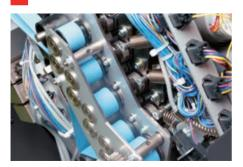
Flexible cross couplings are employed for consistent drive of the fold rollers, even with thick paper or complex folds, and accurate folding performance over the life of the machine. Horizon's unique belt drive system provides reliable, quiet operation.
