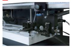
Table Guide Position (Auto for 408F and 406F) A newly designed suction head and feeding system enables consistent feeding. The innovative suction head and assist air provide accurate sheet separation and pick-up. Blowing air volume and height of the suction head can be adjusted according to sheet conditions for stable feeding of a wide variety of sheets.
