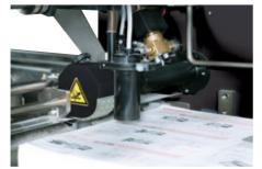
Quality polyurethane rotor provides high speed feeding without scratching. Feed timing and feed interval can be adjusted through the touchscreen. For small size stacks, the feeding operation can be done using only the feed rotor for stable feeding.
