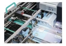
The hold-down roller sets to the proper position to prevent the sheet from bouncing back after hitting the knife stopper. The roller position is automatically adjusted when the sheet or fold pattern is changed.
