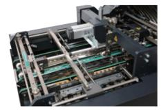
Newly designed rigid and durable knife unit provides consistent quality knife folding. No need to open the knife cover for setup. The entire setup, such as installing the stopper guide, knife angle adjustment and hold down roller position is automated.
