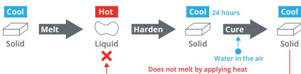
Polyurethane Reactive, also called PUR, is a popular due to its superior binding strength and ecofriendliness.
