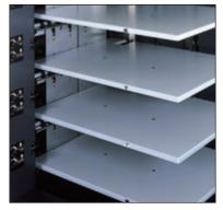
The high capacity feed stations provide maximum production in between re-loads. Accurate feeding is maintained by the easy accessible paper feed controls. Each bin raises automatically to the correct height according to the quality and weight of paper being used. Ruffling and top sheet separation air are easily adjusted at each station to insure smooth feeding of even the most difficult stocks. Absolutely no tools are required.
