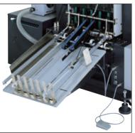
This tray was designed specifically to handle difficult-toalign papers such as NCR paper, or those sheets with spot carbon. In order to assure a perfectly aligned stack of collated sets, the jogger, run by an independent motor, vibrates the sets into place. The tray also descends automatically as it receives the collated sets. To reset the jogger receiving tray and continue operation, simply push the foot pedal.
