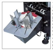
This tray automatically swings 30 degrees after delivery of each collated sequence, making it the perfect tray for jobs such as multi-page booklets. The receiving guides may be adjusted according to the scales provided, allowing for exact receipt of the collated sets. The tray descends automatically as its delivered pile increases. Maximum paper size for this tray is 470 mm x 318 mm / 18.5" x 12.5".
