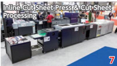
Inline system with the CANON's imagePRESS C810 and our SmartSlitter. The connected CSD-40SMSL Card Stacker allows for the precise stacking with accurate count. To synchronize with the speed of digital press and SmartSlitter, the SBM-100 universal buffering module is connected.
