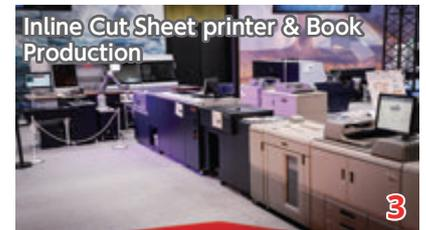
This solution enables variable book production with no operator makereadies. Two presses (one for book blocks and one for cover sheets) are connected inline, with the cover sheets being printed based on book-block contents and then automatically fed into a binder. Book blocks are processed with our SmartSlitter and then fed into the binder with a robotic arm.
