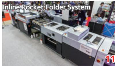
This inline system features our rotary-die cutting, gluing unit, and buckle folder to make pocket folders with environmentally friendly materials.
