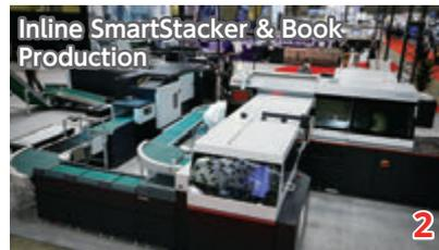
This is our inline book production solution that processes B2 printed sheet into perfect bound books. An AGV brings pallets loaded with B2 printed sheets to our SmartStacker infeed section for automated loading. The SmartStacker is equipped with inspection devices by DAC ENGINEERING for high-level quality control.
