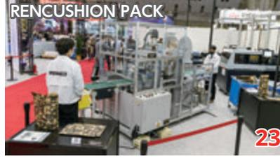
This is the automated packaging system RENCUSHION PACK for all-paper, cushion envelope packaging that eliminates the need for adhesives and bubble wrap. The RFID tags are planted in both hard and soft cover books in our demonstration for appealing the use of scanned data for address printing, progress checking, etc.
