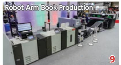
This print-to-book production solution features inline robotic feeding to allow for continuous production. Book blocks are printed by the Riso's VALEZUS T2200 digital press, fed into our single clamp perfect binder with a robotic arm, and then finished with our three-side trimmer.
