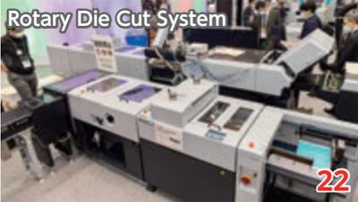
The system is configured with FFU-N4055 sheet feeder, RD-N4055DM rotary die cutter, and SPC-N4055 separator connected with the stacker & delivery unit (under development). This stacker & delivery unit combines the several stacks into one before delivery for the smooth picking operation.
