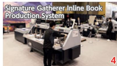
This solution is designed to produce books from offset-printed signatures and features our gatherer, book block feeder, 4-clamp perfect binder and three-side trimmer all connected inline. Palletized signatures will be transported by an AGV from the Folder with Palletizing Robot System.
