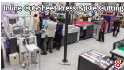
This system connected with the Konica Minolta's AccurioPress C14000 allows for business card production in one pass. The cut alignment and print quality is inspected by DAC Engineering's Preinity scanners. The robot-hand banding section (under development) is equipped for further automation of business card production.
