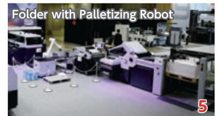
This B1-to-signature production system eliminates all manual labor involved with transportation, loading, and palletizing by utilizing an AGV and robotic arm.
