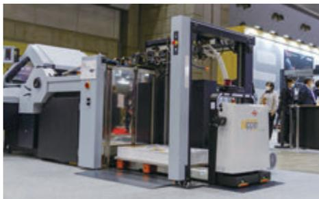
The sheets (A4 duplex 16-page) were printed by RMGT 970PF-8 at the RYOBHI MHI Graphic Technology Ltd. and delivered to the feeder of Folder with Palletizing Robot system by Nipper (AGV).
