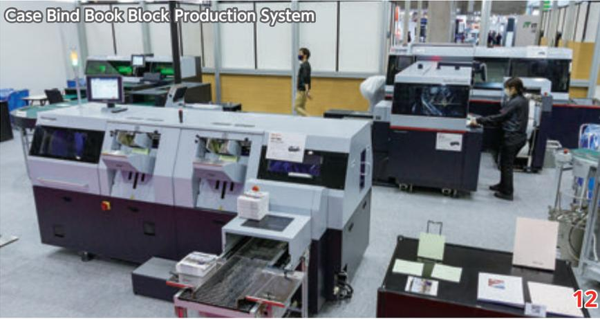
This inline solution allows for high-mix, low-volume case preparation from any type of book block by integrating our end sheet feeder, loose-sheet book block feeder, perfect binder, gauze applicator, and trimmer into one system. The RFID tags are planted in both hard and soft cover books in our demonstration for appealing the use of scanned data for address printing, progress checking, etc.
