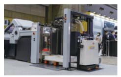
The sheets (A4 duplex 16-page) were printed by RMGT 970PF-8 at the RYOBI MHI Graphic Technology Ltd. and delivered to the feeder of Folder with Palletizing Robot system by Nipper (AGV).
