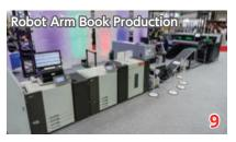
This print-to-book production solution features inline robotic feeding to allow for continuous production. Book blocks are printed by the Riso's VALEZUS T2200 digital press, fed into our single clamp perfect binder with a robotic arm, and then finished with our threeside trimmer.
